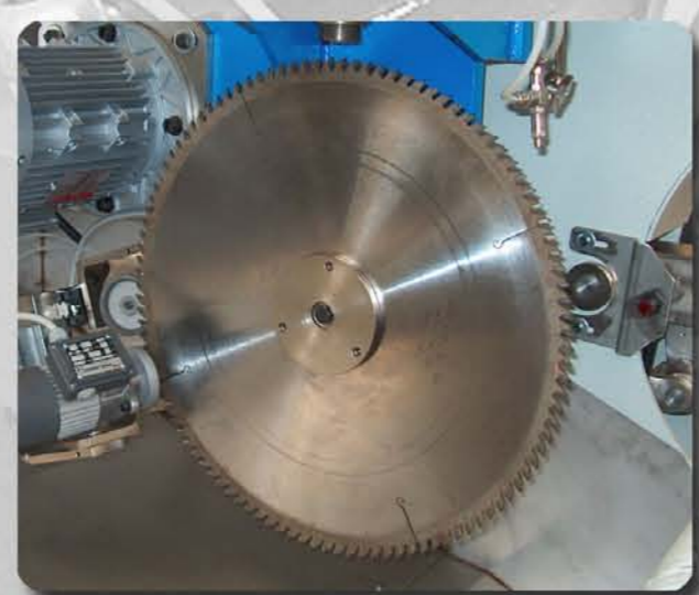
Lama a sega per materiali rigidi Serrated blade for rigid materials
