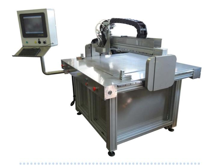
Machine for hot melt adhesive deposition with 2 controlled axes .
